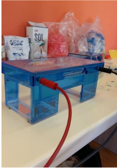
Picture 8. Gel electrophoresis used in the experiment
