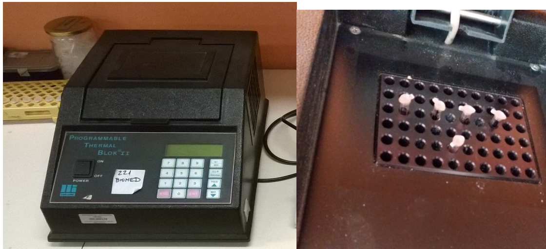
Figure 2: The PCR cyciler we used for our projects. Picture left represents the whole machine and the picture right are our samples prepared for the PCR process.
