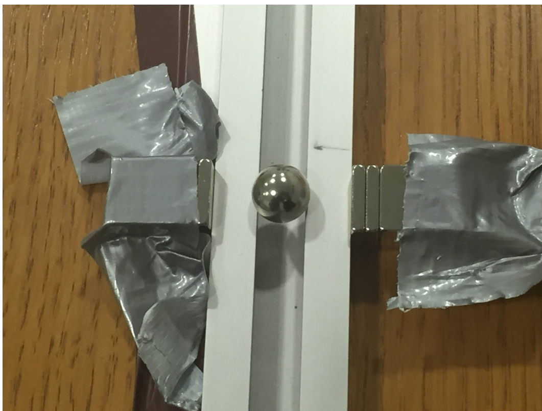
Figure 3. Configuration of magnets for trapping without the acceleration stage.
