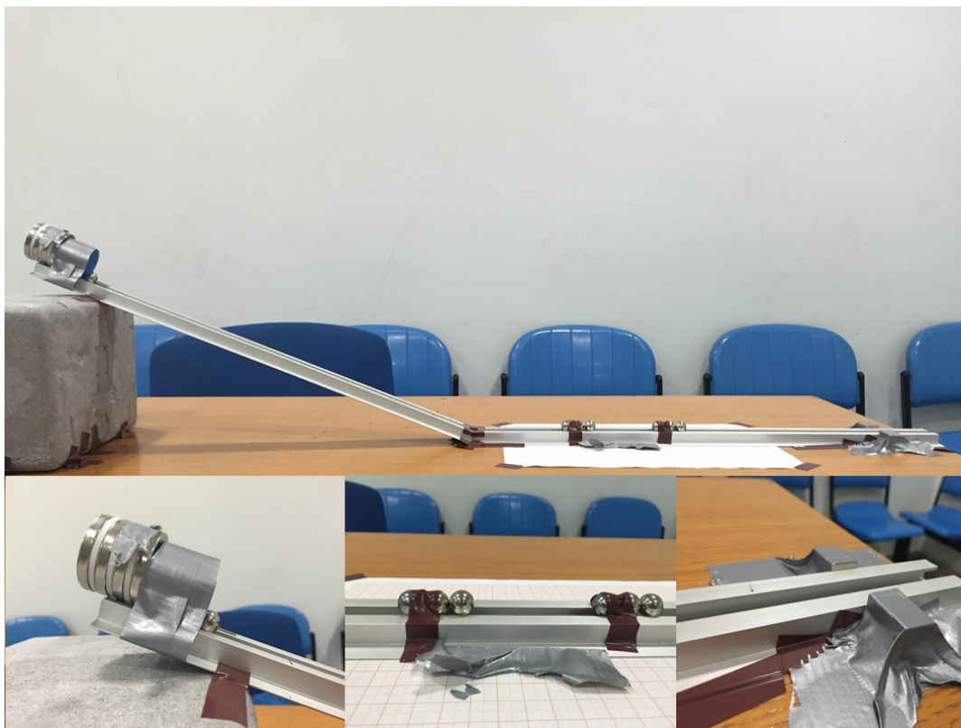
Figure 1. Photograph of experimental setup with the release mechanism, accelerator system, and deceleration and trapping magnets in separate panels.
