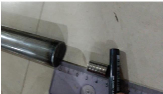
Figure 5. Estimation of unknown permeability of two different ferromagnetic rods. The rod with higher permeability is attracted more by a static magnet and is, therefore, chosen as a core for electromagnet.
