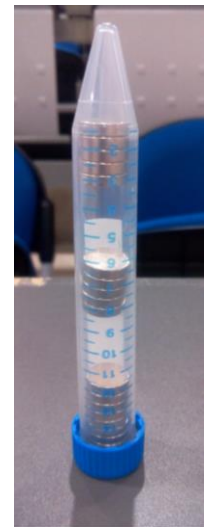
Figure 2. Magnetic field created by two static magnets that repel each other (left). Lab experiment done by applying the aforementioned principle. A container is needed to prevent magnets from spinning (right).
