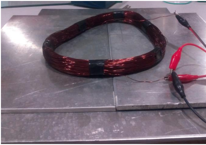
Figure 11. Hoverboard formed of electromagnet as levitating object, above four symmetrically placed aluminium plates. It is important to maintain a small gap between two adjacent plates in order to keep the levitating object firmly in place.
