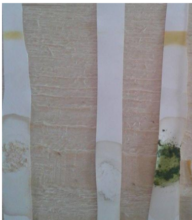
Fig. 8 - Results of chromatography. Left - carrots, 1st type of paper. Middle - carrots, 2nd type of paper. Right - spinach, 1st type of
